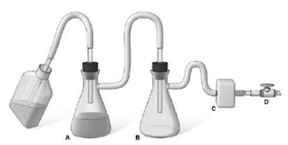
Aspiration flask (A) – collect contaminated fluids (e.g., tissue culture media) into appropriate disinfectant (e.g., 10% bleach); Overflow flask (B) – collects overflow fluids and tube submerged on liquid minimizes aerosols; HEPA filter (C) – in-line filter prevents contamination of vacuum; Vacuum line (D) – in-house central vacuum system or vacuum pump.
