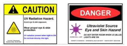
**Eye/Face protection** must be marked with ANSI Z87.1 UV certification (Z87U)
