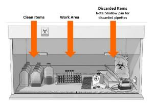
A typical layout for working from the clean to the dirty side within a Class II biosafety cabinet. This arrangement is reversed for left-handed persons.
